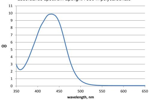
absorbance spectrum Epolight 7830 in polycarbonate
